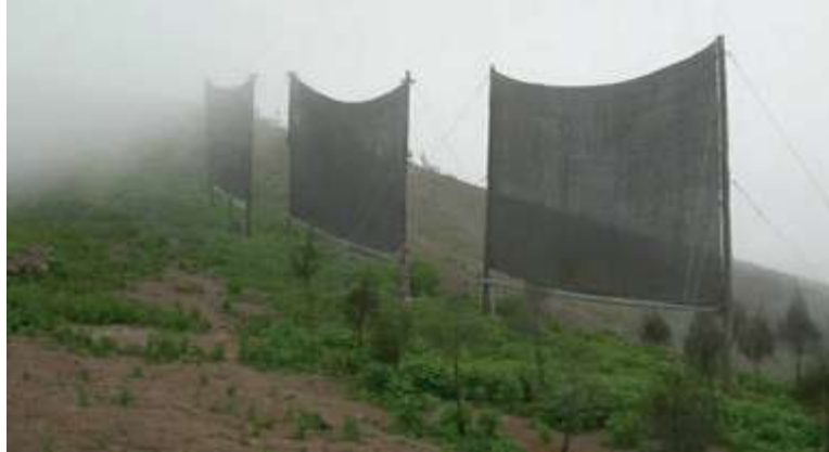
Fig. 2: Fog and dew harvest device.
