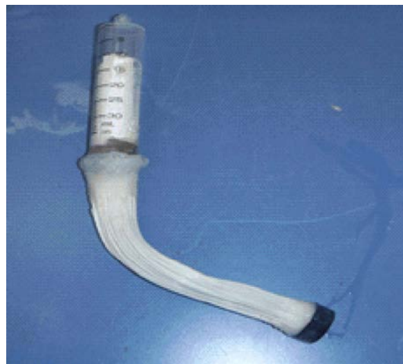
Fig. 1: Handmade micro-filter for greywater filtration
